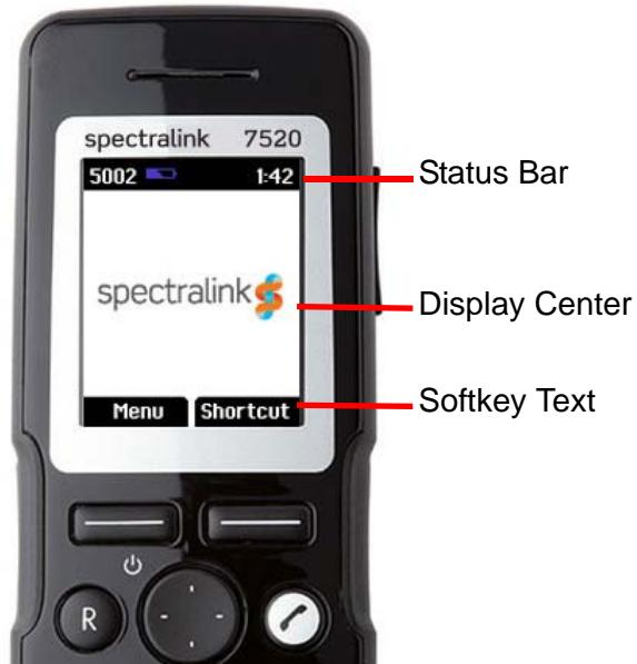
The display is divided in three parts: Status bar, Display center and Softkey Text (see figure above).
